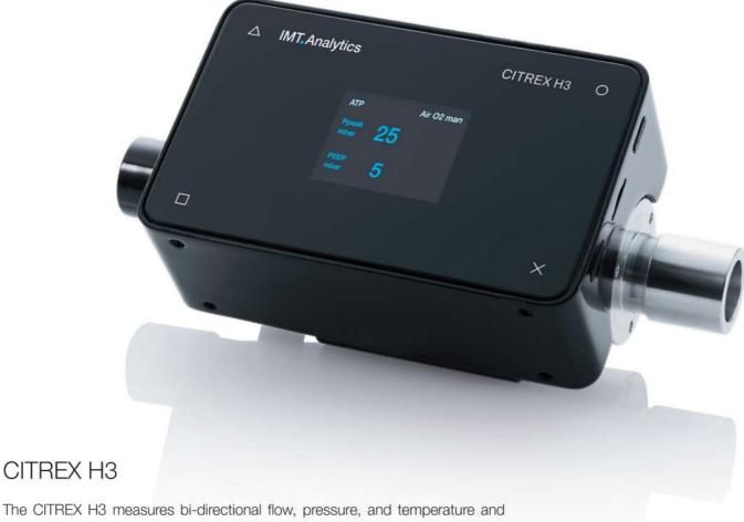
The CITREX H3 measures bi-directional flow, pressure, and temperature and optionally oxygen concentration. Gas flow is pressure, temperature and humidity compensated and can be displayed in many different gas standards. This brings additional flexibility to the user. With an internal battery, the CITREX H3 can perform measurements for many hours on a single charge. The USB power connector allows for simple recharging at any time.
